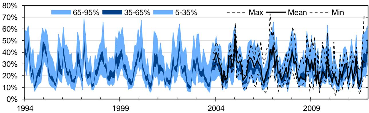
**Figure 2: The distribution of monthly average load factor across the 120 wind sites, comparing simulation (shaded areas) with measured historical output (lines).**
