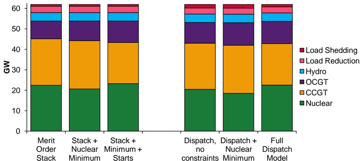
**Figure 6: Optimal capacity mixes calculated by each model.**
