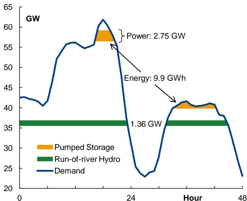
**Figure 5: Demonstration of the heuristic for allocating hydro resource.**
