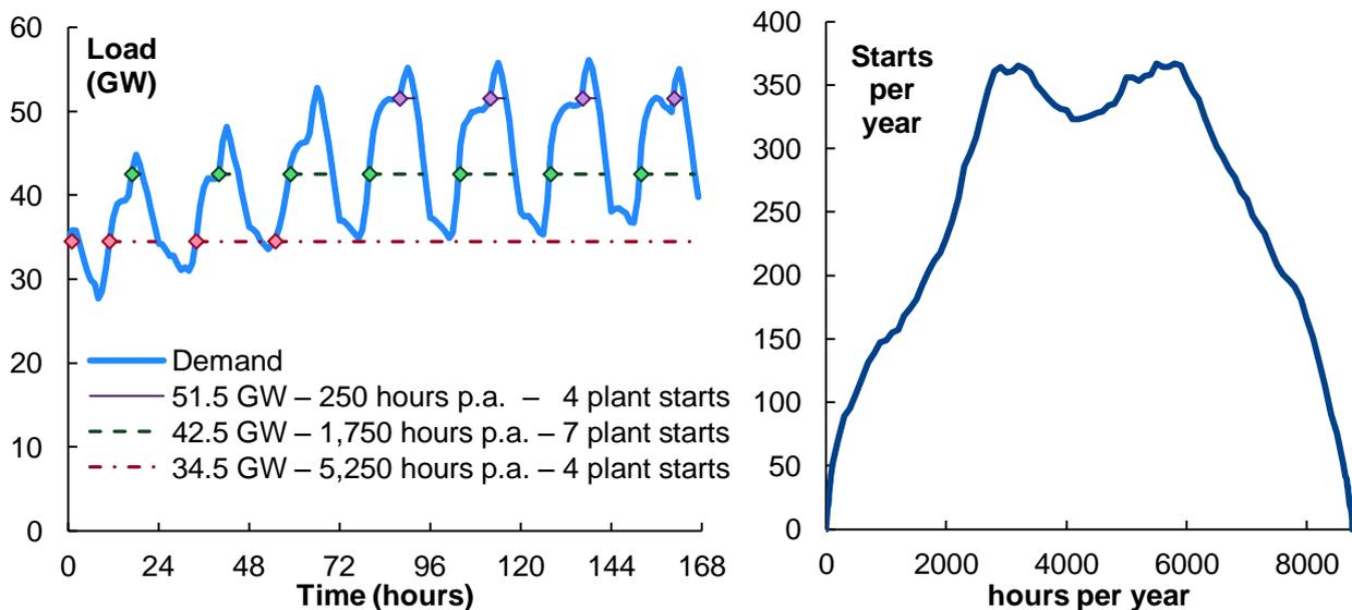
**Figure 3: Demonstrating a simple algorithm for calculating the number of start-ups for different levels of plant.**
