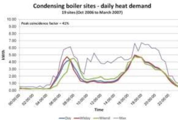
Figure 9 - Condensing boiler daily heat demand
