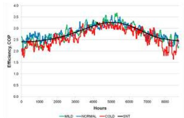
Figure 11 - ASHP hourly annual efficiency for temperature scenarios<sup>3</sup>
