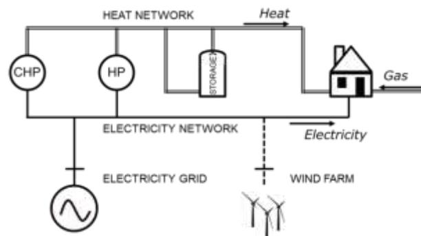
Figure 22 – Integrated heat and electricity model
