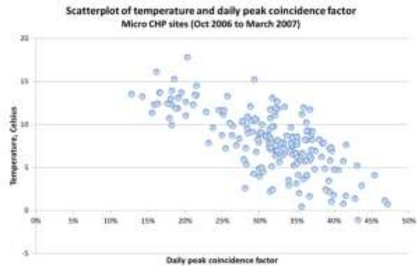
Figure 10 - Scatter plot of temperature and daily peak coincidence factor
