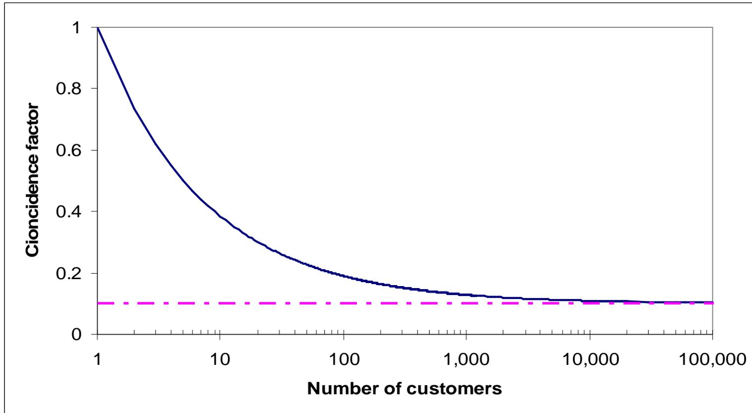
**Peak demand of a typical house is about 10kW: to supply 10,000 houses we do NOT need 100,000kW of supply capacity but ONLY about 10,000kW due to load diversity**
