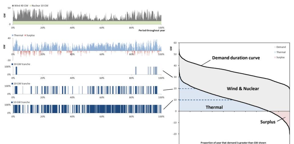
**Figure 3:** Illustrative operating patterns for thermal plants operating at 10 GW, 20 GW and 30 GW tranches in merit order, (left) and duration curves for 40 GW wind and 10 GW nuclear capacity for the year 2000 (right).
