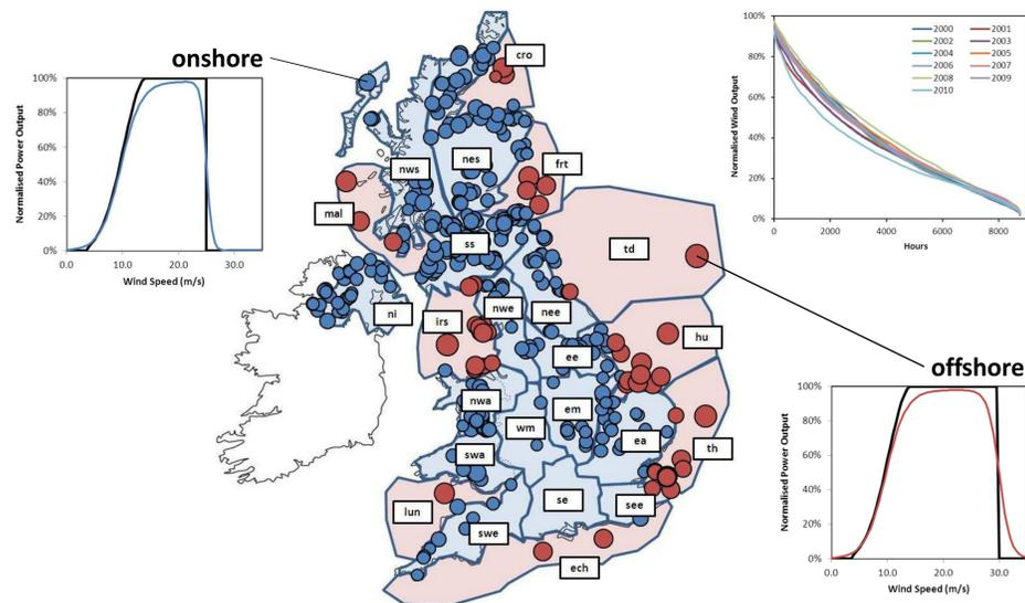
**Figure 1:** Aggregate power output curves were used to convert wind speeds for 337 onshore and 49 offshore wind sites and (top right) the non-chronological normalised wind output for 11 historic years illustrates inter-annual wind output variability [1][2].
