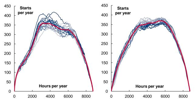
Figure 4: Average number of plant start-ups for the GB system from 1994–2011 (left), and for the New England system from 1980–2011 (right). Individual years' data is shown in blue, with the period average highlighted in red.
