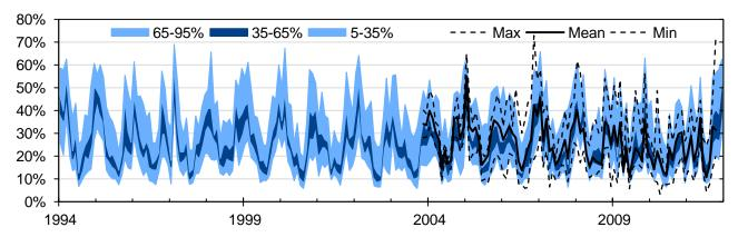
Figure 2: The distribution of monthly average load factor across the 120 wind sites, comparing simulation (shaded areas) with measured historical output (lines).
