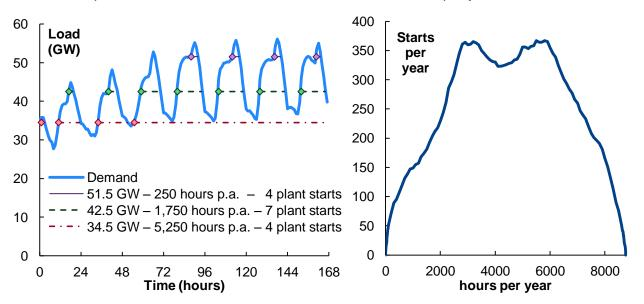
Figure 3: Demonstrating a simple algorithm for calculating the number of start-ups for different levels of plant.
