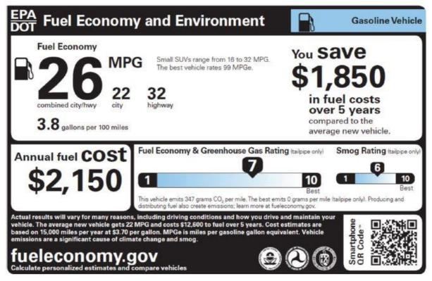
Figure 4 U.S. Environmental Protection Agency Fuel Economy and Environment Label for Gasoline Vehicles (from Ungemach et al 2017)
