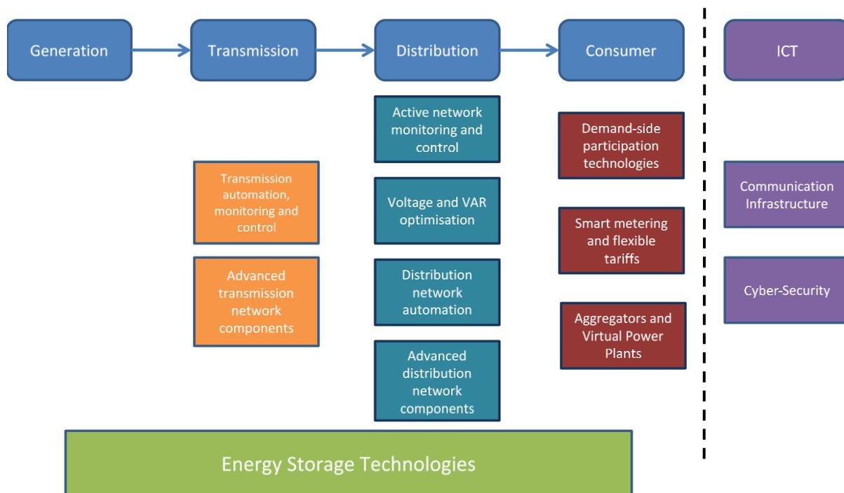
Figure 1: Technology Clusters in a Typical Smart Grid System
