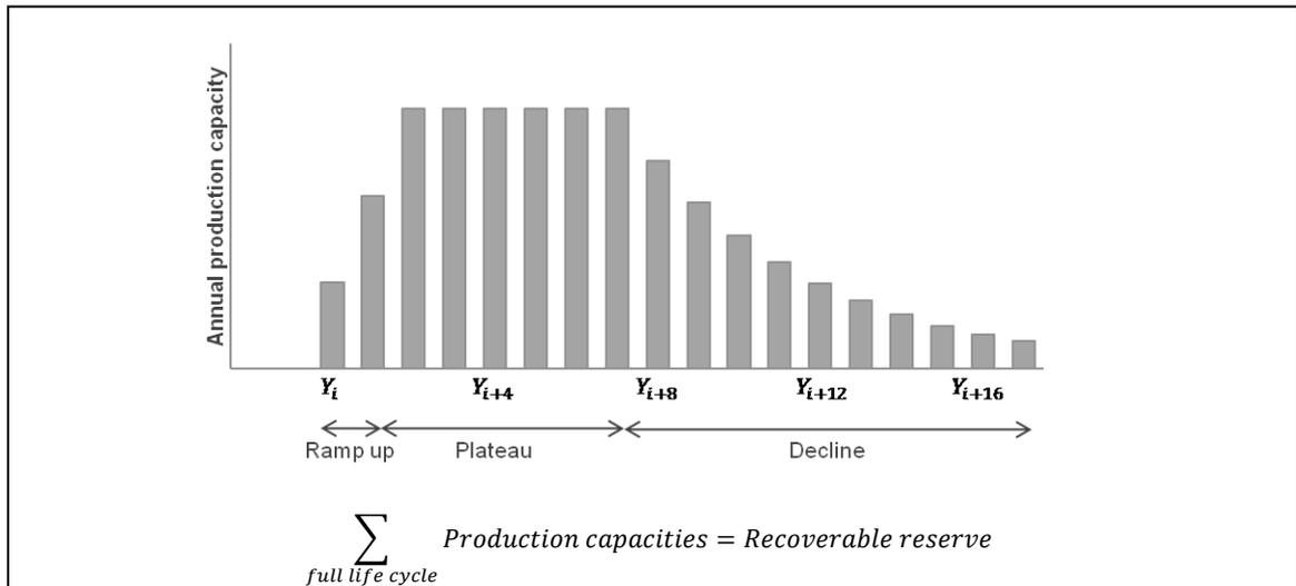
**Figure 4 NG schematic production profile**
